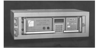
As the aggregate hits the meter, the moisture content is measured and digitally displayed.
